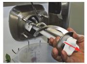
**5. Remove** the beater from the cylinder. (**Be careful** not to drop the scraper blades onto the ground.)
