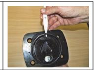
**3. Remove** the gasket on the back of the ice cream head.
