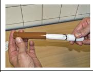
**6. Assemble** the outer feed pipe and inner feed pipe.
