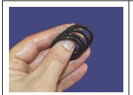
**1. Lubricate** the O rings for the piston and the mix feed pipe.
