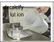
**1. Fill** the mix tank completely with decalcify solution.
