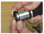
**2. Fit** the two O rings on the piston.
