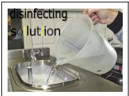
**1. Fill** the mix tank completely with disinfecting solution.
