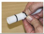
**5. Fit** the two O rings on the iner mix feed pipe.
