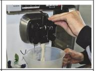
**3. Drain** all the disinfecting solution out of the machine.
