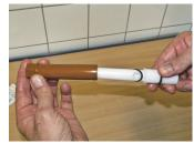
**5. Disassemble** the outer and inner pipe of the mix feed pipe.
