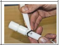
**6. Remove** the two O rings from the mix feed pipe.
