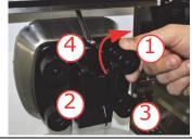
**9.** Loosely **tighten** the four bolts in the sequence shown. Then tighten firmly by hand following the same sequence.
