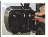
**1. Remove** the locking pin from the dispensing handle.
